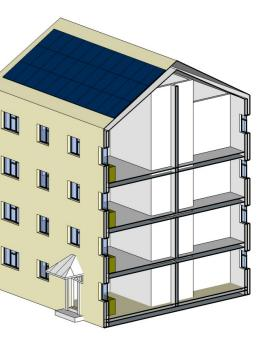
Retrofitted to achieve net zero carbon: Heat pumps, 150+mm of continuous insulation to floors, walls and roof, very good double or triple glazing, excellent levels of airtightness and mechanical ventilation with heat recovery. Full-size photovoltaic array fitted with high efficiency modules and microinverters. Space heat demand of around 40kWh/m<sup>2</sup>/year. Net
