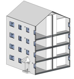
Baseline block of flats: Gas boilers or electric heating, little insulation, single or poor double glazing, poor airtightness and uncontrolled ventilation through gaps in the building fabric. Space heat demand of around 160kWh/m<sup>2</sup>/year.
